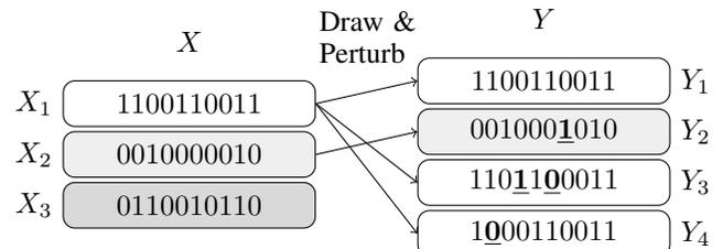
Fig. 1: Exemplary realization of the DNA storage channel with  $M = 3$  and  $N = 4$ . Shades highlight the origin of the received sequences. This origin is however *unknown* to the receiver.
