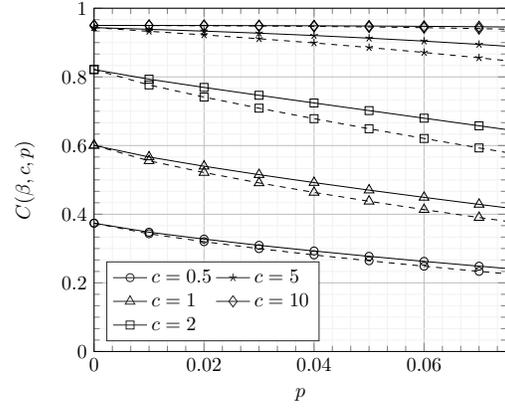
Fig. 2: Capacity of the noisy drawing channel for different values of  $c$ , over a range of error probabilities  $p$ , with  $\beta = \frac{1}{20}$ . The dashed lines show achievable rates for suboptimal majority vote decoding.
