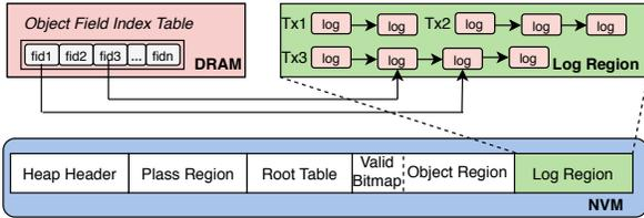
Figure 2: The shared NVM heap structure in UNIHEAP.
