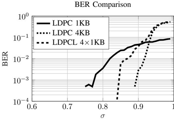
Fig. 1. BER comparison between three rate-half codes: an LDPC code with block length  $n = 4KB$ ; an LDPC code with same degree distributions, but shorter block length  $n = 1KB$ ; a random-access LDPCL code with  $M = 4$  sub-blocks with length  $n = 1KB$  each.
