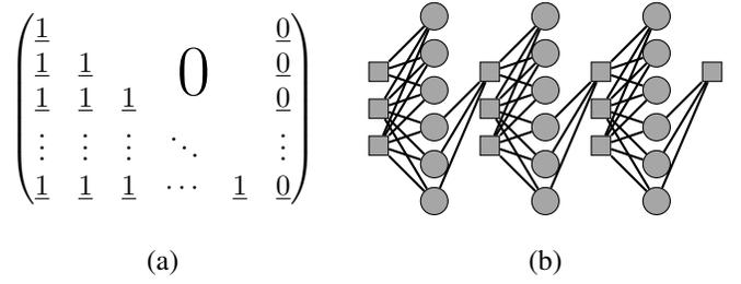
Fig. 2. (a) Matrix  $A_1$  from Construction 1. (b) The  $(3, 6, 1)$  SC-LDPCL protograph with  $M = 3$  SBs.
