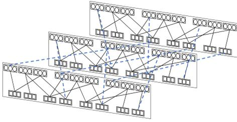
Fig. 1: An MD-SC code constructed by rewiring  $\mathcal{T} = 1$  group of connections per replica. Constituent SC codes have parameters  $\kappa = 3$ ,  $\gamma = 2$ ,  $z = 3$ ,  $m = 1$ , and  $L = 3$ . Circles (resp., squares) represent VNs (resp., CNs). Each line represents a group of connections. Rewired connections are shown in dashed blue lines.
