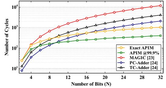
Fig. 2. Performance comparison of the proposed design with previous work for addition of  $N$  operands, each sized  $N$  bits.
