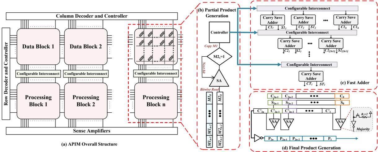
Fig. 1. (a) The overall structure of APIM consisting of several data and processing blocks. (b) the APIM controller and parallel product generator. (c) Fast adder three structure consisting of Carry save adder and configurable interconnects. (d) Final product generator to ripple the carry bits of tree structure.
